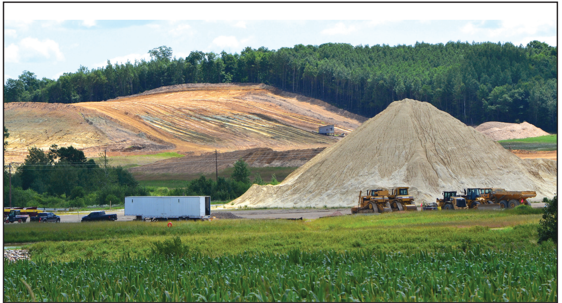
Frac sand mining operations like this one in western Wisconsin rely on removing topsoil — called “overburden” by the industry — to get access to the silica sand. (LSP Photo)
