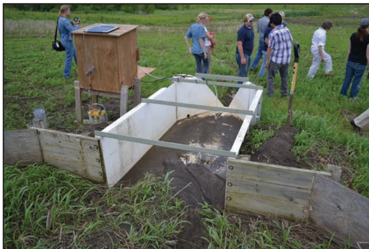
Flumes like this are designed to measure how much soil is eroding from fields being studied. This one, which lies at the bottom of a slope planted to no-till soybeans but no prairie strips, is full of silt. (LSP photo)
