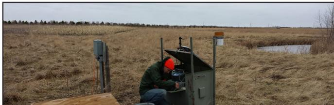
**Figure 6:** Paul Wymar adjusting sampler to monitor tile line drainage from a Shakopee Creek corn-soybean field. (Paul Wymar photo)
