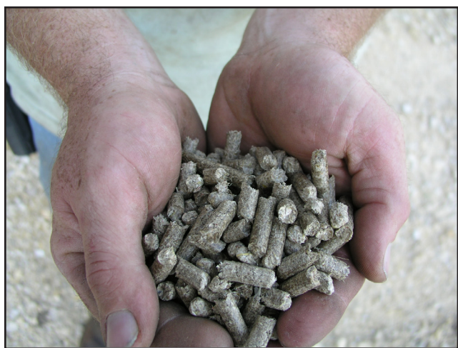
The Kreidermachers are experimenting with processing plant material into dense pellets that can be stored, transported and burned efficiently. (LSP photo)
