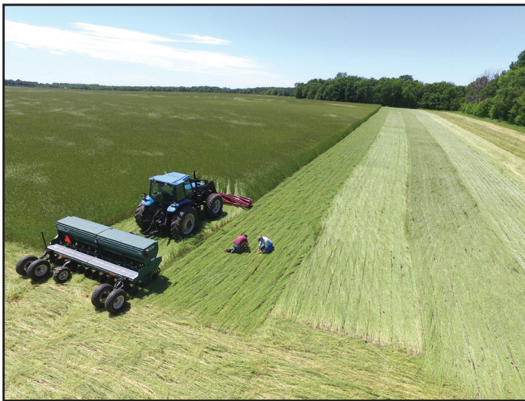
The roller crimper system, which the Jovaags use in conjunction with cover crops, is helping build aggregate structure on previously damaged soils. (Photo by Paul Hunter, Mower County SWCD)
