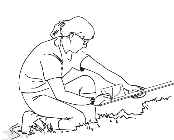
Figure 8a: Measuring bank angle with protractor and yardstick.
